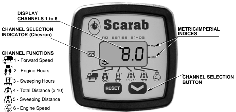
Fig. 15 The RDS Sweeper Monitor
